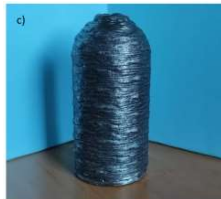
Figure 3. Example of hollow cylinder manufactured by WAAM on a bottom composed of spiral type layers such as that of Fig. 2.
