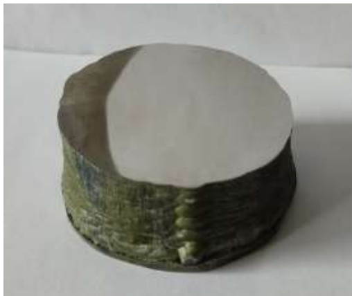
Figure 5: Cross-section of a part after HIP of powder in a cylinder manufactured by WAAM.
